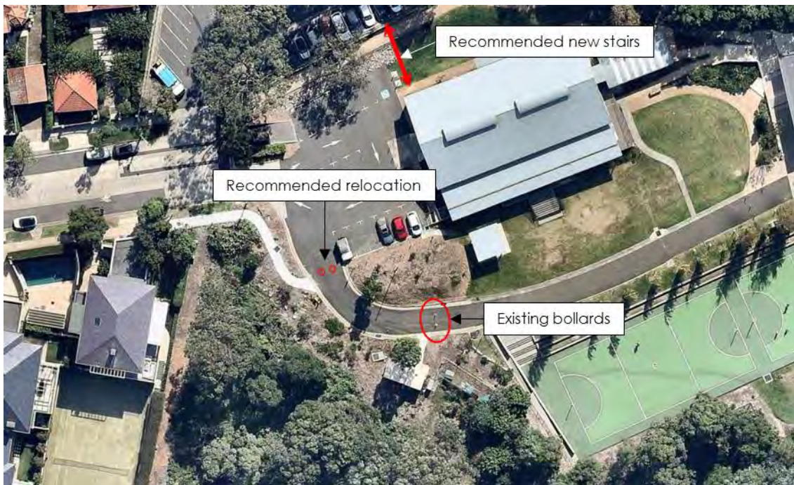
Figure 3.4: Recommended new stairs and relocation of bollards
