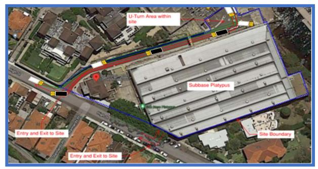
Figure 7. Showing the ability to perform a U turn at the bottom of Platypus Lane. (The maximum length of trucks will be 8936mm)
