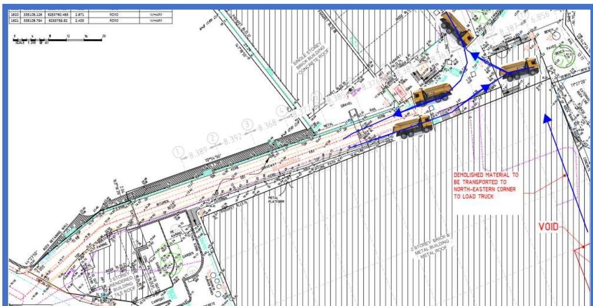
**Figure 6. Showing the ability for construction vehicles to manoeuvre within Platypus Lane to exit in a forward direction. (The maximum length of trucks will be 8936mm)**
